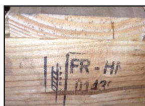
Unacceptable markings (illegible)
